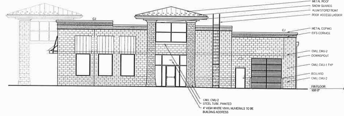
33 A2.1 RIGHT BUILDING ELEVATION SCALE: 1/8" = 1'-0"
